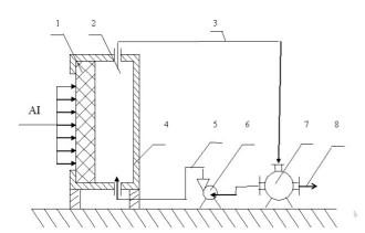
Fig. 1. Scheme of the reactor's cell: 1 - GDE.; 2 - reactor chamber; 3 - waste solution line; 4 - reactor; 5 - solution supply line; 6 - peristaltic pump; 7 - solution tank; 8 - sampling line.
