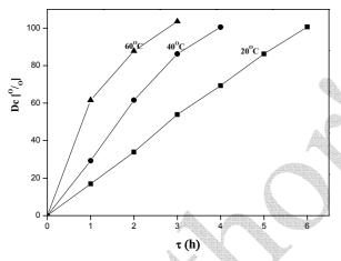
Fig. 6. Relationships between degree of conversion and time on stream at different temperatures for Ni(OH)<sub>2</sub> catalyst on GDE: SGDE = 200 cm<sup>2</sup>; T = 20, 40 and 60°C; electrolyte: 15 g S<sup>2-</sup>·l<sup>-1</sup> + 0.25 N NaOH + O<sub>2</sub> (Air); flow rate  $v_r$  = 24.15 cm<sup>3</sup>·min<sup>-1</sup>.
