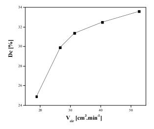
Fig. 2. Relationship between rate of sulphide oxidation by oxygen and flow rate of solution;  $T = 20^{\circ}\text{C}$ ; electrolyte: 15 g S<sup>2-</sup>·l<sup>-1</sup> + 0.25 N NaOH; non-modified GDE SGDE = 200 cm<sup>2</sup>.
