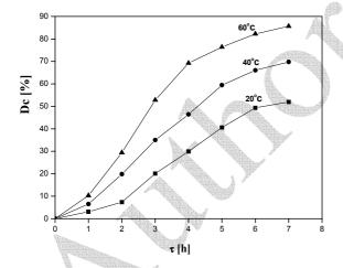
Fig. 3. Relationships between degree of conversion and time on stream at different temperatures: T = 20, 40 and 60°C; electrolyte: 15 g S<sup>2-</sup>·l<sup>-1</sup> + 0.25 N NaOH + O<sub>2</sub> (Air); non-modified GDE; SGDE = 200 cm<sup>2</sup>; flow rate  $v_r = 24.15 \text{ cm}^3 \cdot \text{min}^{-1}$ .
