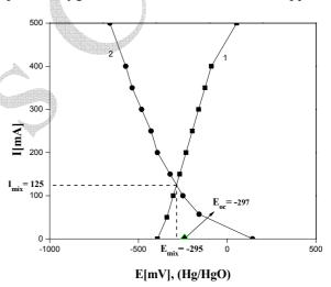
Fig. 4. Partial polarization curves:  $T = 20^{\circ}\text{C}$ ; non-modified GDE;  $v_r = 24.15 \text{ cm}^3 \cdot \text{min}^{-1}$ ; SGDE =  $200 \text{ cm}^2$ ; cathodic curve ( $\blacksquare$ ) -  $15 \text{ g S}^{2-}\text{I}^{-1} + 0.25 \text{ N NaOH} + \text{Ar}$ ; anodic curve ( $\bullet$ ) -  $0.25 \text{ N NaOH} + \text{O}_2$  (Air);  $E_{0c}$  ( $\triangle$ ) -  $15 \text{ g S}^{2-}\text{I}^{-1} + 0.25 \text{ N NaOH} + \text{O}_2$  (Air).
