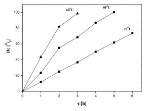
Fig. 5. Relationships between degree of conversion and time on stream at different temperatures for CoPc(SO<sub>3</sub>H)] catalyst on GDE: SGDE = 200 cm<sup>2</sup>; T = 20, 40 and 60°C; electrolyte: 15 g S<sup>2-</sup>·l<sup>-1</sup> + 0.25 N NaOH + O<sub>2</sub> (Air); flow rate  $v_r = 24.15$  cm<sup>3</sup>·min<sup>-1</sup>.
