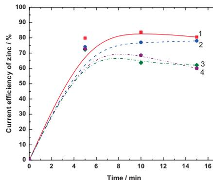
**Figure 3.** Current efficiency of Zn deposition at potential (vs. SSE): -1.600 V as a function of time: 1)  $\text{Zn}^{2+}$ -50 g/L and  $\text{H}_2\text{SO}_4$ -130 g/L, 2)  $\text{Zn}^{2+}$ -50 g/L,  $\text{H}_2\text{SO}_4$ -130 g/L and  $\text{Cu}^{2+}$ -50 mg/L, 3)  $\text{Zn}^{2+}$ -50 g/L,  $\text{H}_2\text{SO}_4$ -130 g/L and  $\text{Cu}^{2+}$ -100 mg/L, 4)  $\text{Zn}^{2+}$ -50 g/L,  $\text{H}_2\text{SO}_4$ -130 g/L,  $\text{Cu}^{2+}$ -100 mg/L and  $\text{Fe}^{2+}$ -100 mg/L.
