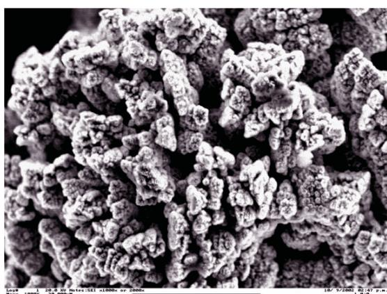
**Figure 5.** SEM micrograph of Zn, containing 2.4 wt.% Cu and 0.25 wt.% Fe. Electrolyte:  $Zn^{2+}$  - 50 g/L,  $H_2SO_4$  - 130 g/L,  $Cu^{2+}$  - 200 mg/L and  $Fe^{2+}$  - 200 mg/L. Deposition potential (vs. SSE): -1.600 V. Deposition time - 60 min.
