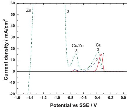
**Figure 1.** Anodic peaks of dissolution of Cu layers, deposited in an electrolyte, containing  $\text{Zn}^{2+} - 50 \text{ g/L}$ ,  $\text{H}_2\text{SO}_4 - 130 \text{ g/L}$  and  $\text{Cu}^{2+} - 50 \text{ mg/L}$  on an Al cathode at potentials (vs. SSE): 1)  $-1.330 \text{ V}$ , 2)  $-1.430 \text{ V}$ , 3)  $-1.470 \text{ V}$ . Time of deposition -  $15 \text{ min}$ . Scan rate -  $10 \text{ mV/s}$ .
