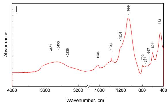
Fig.5. IR absorbance spectra of Ag loaded CL.
