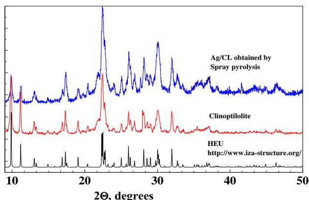
Fig 2. XRD diffractogram of CL, Ag loaded CL and HEU type structure according to zeolite data base atlas.
