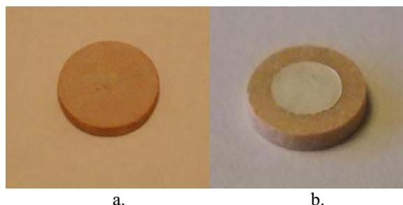
**Fig. 1.** Samples used for electrochemical investigation: (a) sample before the deposition of the electrodes; (b) sample with silver electrodes.
