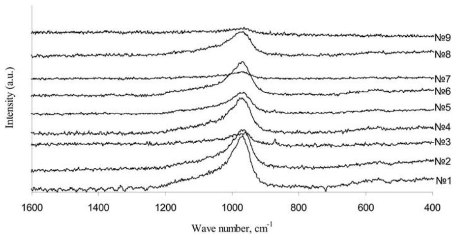
Fig. 3. Raman spectra of the glass samples
