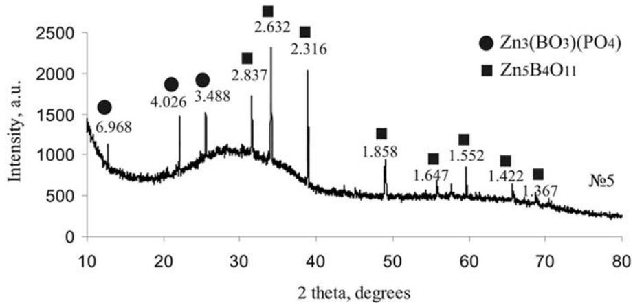
Fig. 2. Powder X-ray diffraction pattern for sample № 5
