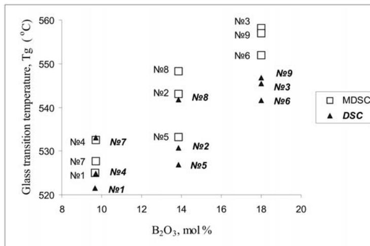
Fig. 5. Dependence of the glass transition temperature obtained by DSC and TMDSC versus the content of B<sub>2</sub>O<sub>3</sub>
