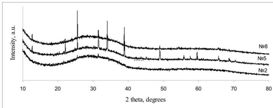
b. Powder X-ray diffraction patterns for samples № 2, 5, 8 ( $B_2O_3:P_2O_5=1:1$ )
