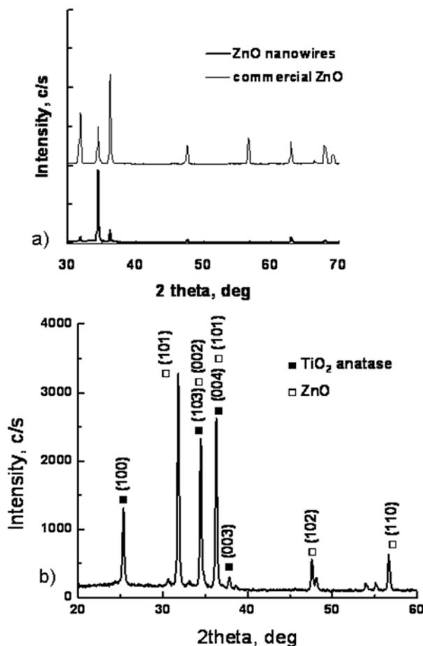
Fig. 4. Comparative XRD patterns of (a) commercial ZnO powder to nanowire ZnO film and (b) XRD pattern of mixed TiO<sub>2</sub>/ZnO film of weight ratio 3:1
