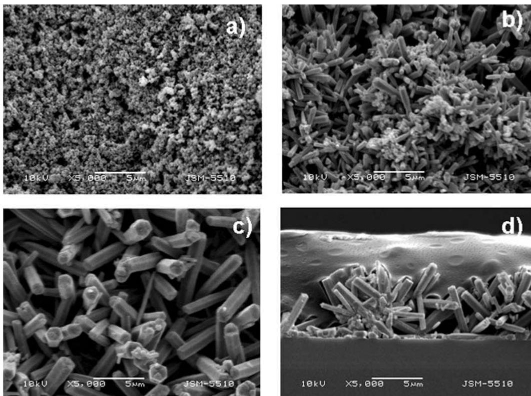
**Fig. 3.** SEM images of TiO<sub>2</sub>/ZnO nanowire arrays: (a), (b), (c) TiO<sub>2</sub>/ZnO arrays (top view) at different magnifications; (d) shows films cross section – TiO<sub>2</sub>/ZnO nanowire array with TiO<sub>2</sub> nanoparticles film on the top
