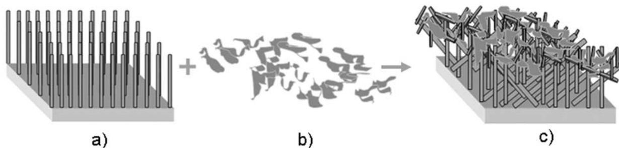
**Fig. 5.** Schematic illustration of (a) ZnO nanowires; (b) TiO<sub>2</sub> suspension in ethanol; (c) ZnO nanowires with TiO<sub>2</sub> nanoparticles
