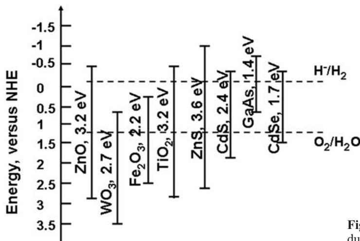
Fig. 1. Band edge positions of common semiconductor photocatalysts (data from [5–7])
