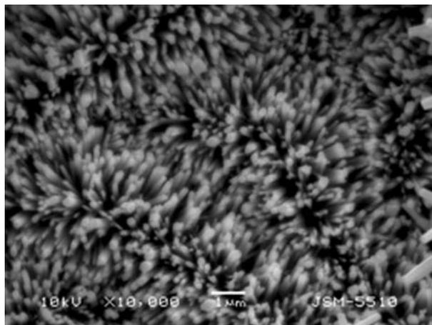
**Fig. 2.** SEM images of top view of the ZnO nanowires
