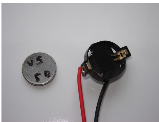
Fig. 5. Li-Air button cell 2032 and holder
