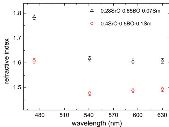
**Fig. 3.** Refractive index values measurements using polarizer-sample-analyzer ellipsometry. The standard deviation is  $\pm 0.001$ .
