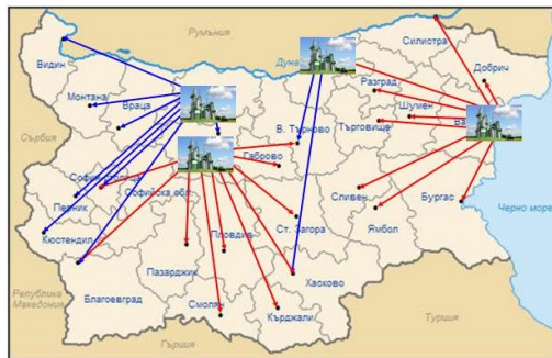
Fig. 5. Optimal BG biodiesel(B100) supply chain configuration in case (a)–Minimum GHG emission for BSC.
