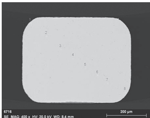
Fig. 4. Scanning electron microscopy image of the cross-section of Posterior part of orthodontic archwire
