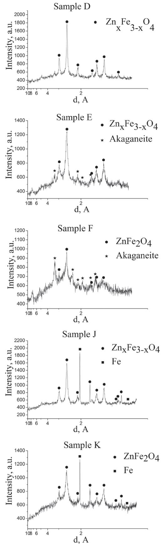
**Fig. 2.** PXR D patterns of synthesized nanosized zinc ferrite-type samples
