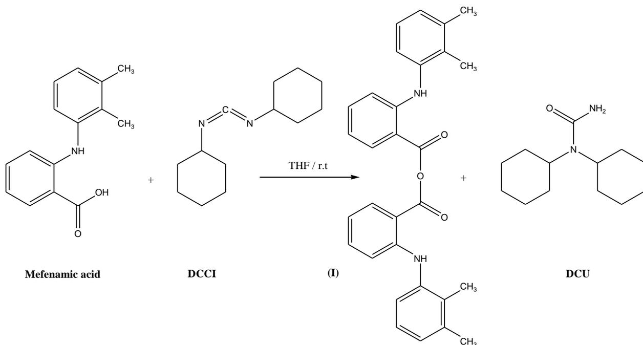
**Scheme 1.** Scheme of the synthesis of intermediate (I)
