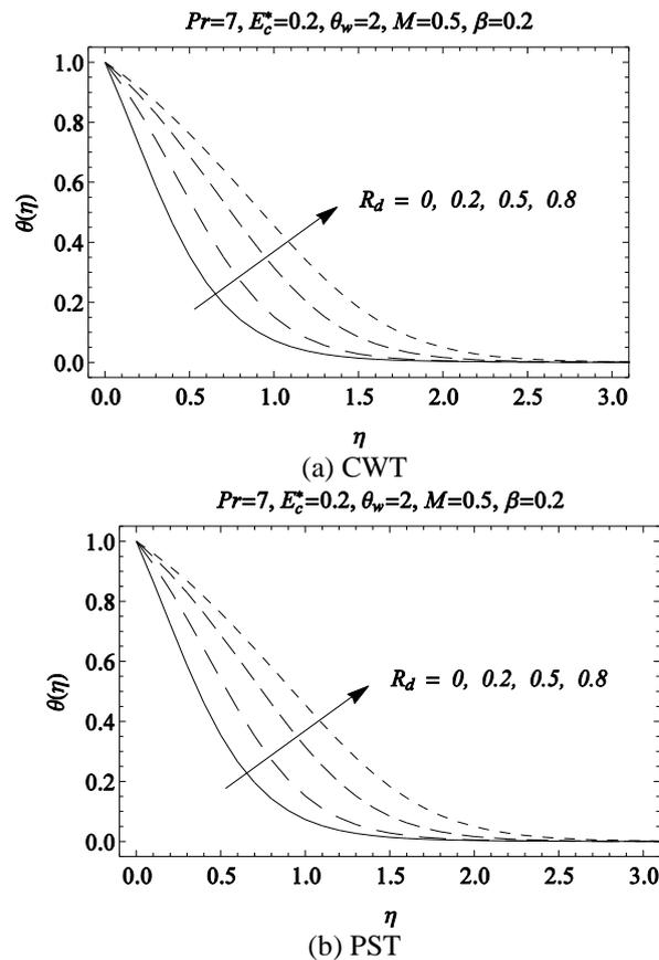
**Fig. 2.** Temperature profiles for different values of the radiation parameter  $R_d$ .
