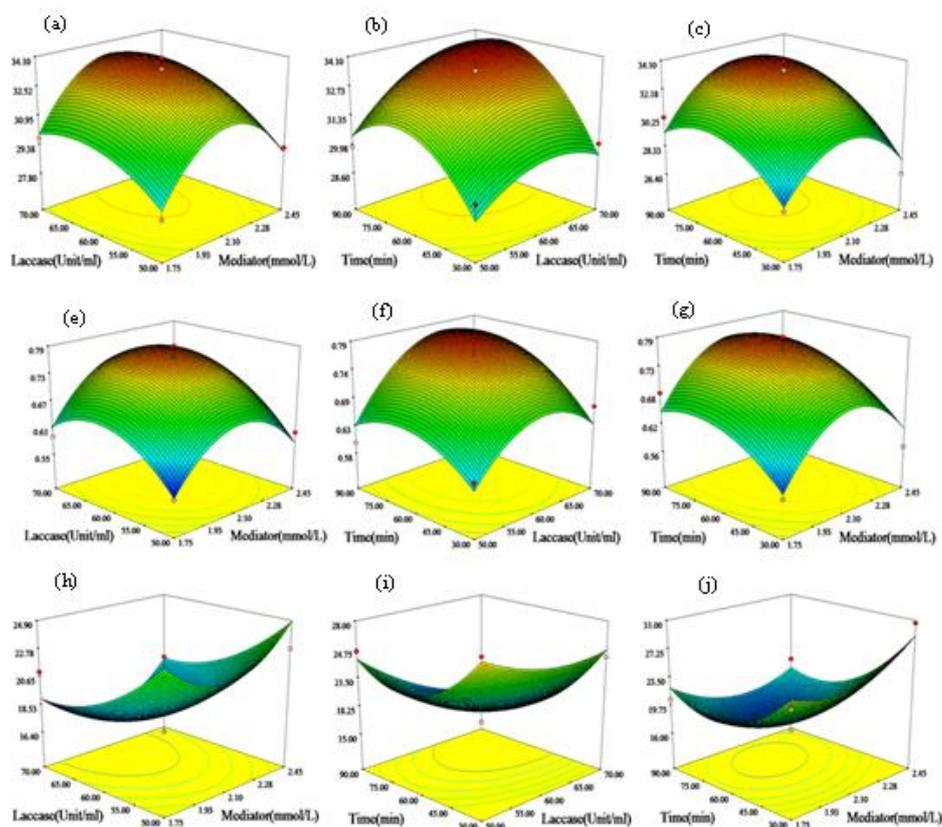
**Fig. 1.** Response surfaces of MOR, IB and WA interacted by laccase, mediator and time
