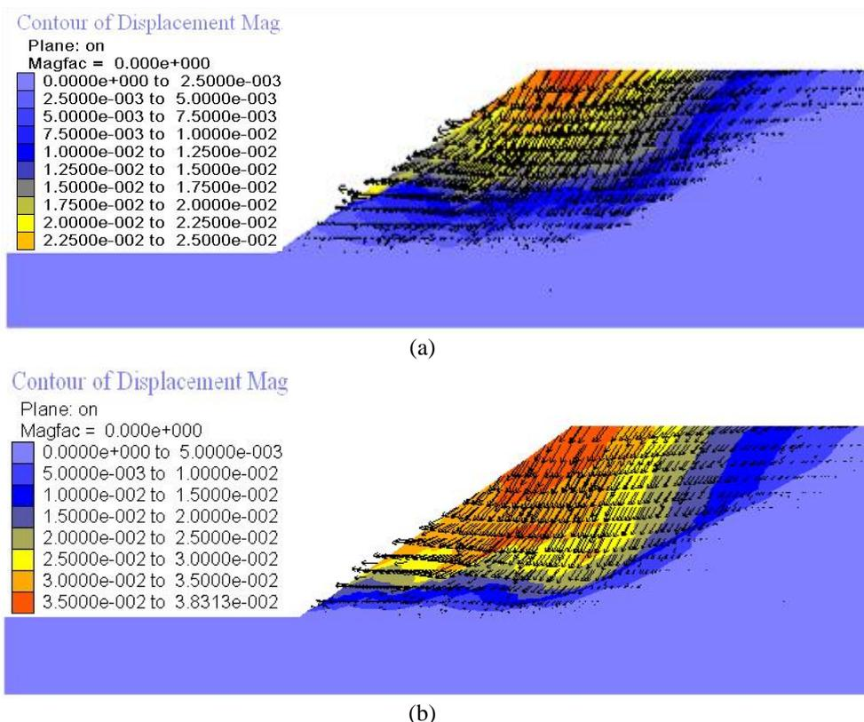
Fig. 6. (a) Displacement vector cloud of Scheme 1; (b) Displacement vector cloud of Scheme 5.
