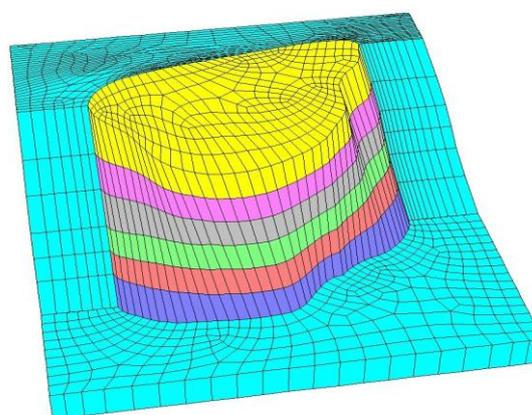
**Fig. 5.** Three-dimensional geological model of the dump.
