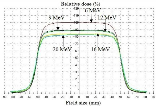
Fig. 4. Crossplane profile curves for all energies – radiation field  $10 \times 10$  cm. (Mephysto 3.0).
