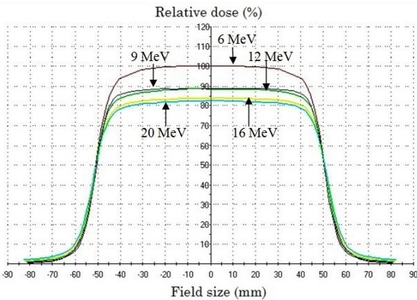
Fig. 3. Inplane profile curves for all energies – radiation field  $10 \times 10$  cm. (Mephysto 3.0).
