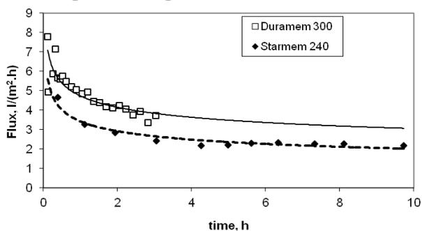
Fig. 1. Measured flux versus time of filtration
