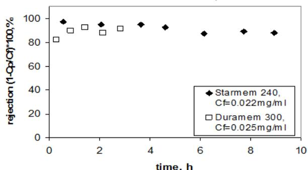
Fig. 2. Measured rejections versus time of filtration
