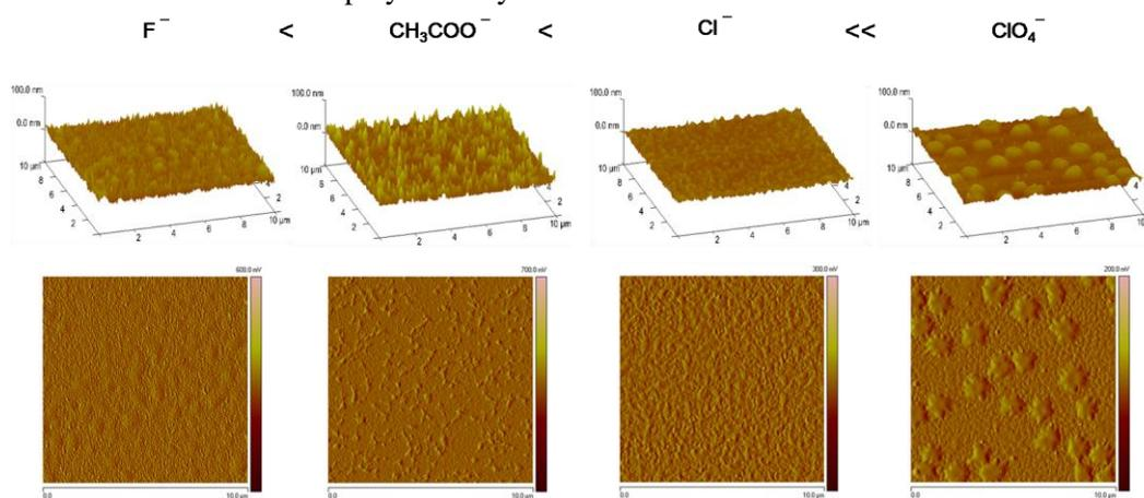
Fig. 2. Typical 3D- (top) and deflection- (bottom) images of (HA/Chi)<sub>5</sub> films on silicon taken by AFM in tapping mode.
