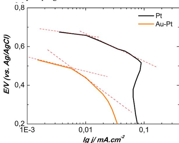
**Figure 5** Quasi steady state polarization curves of ORR of the sputtered catalytic films in 0.5M H<sub>2</sub>SO<sub>4</sub>; scan rate 1 mV.s<sup>-1</sup>.
