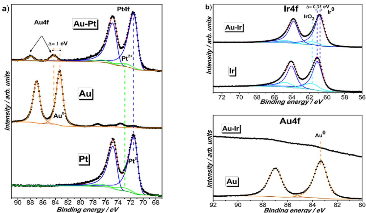
Figure 2. High resolution Au4f-Pt4f (a) and Au4f- Ir4f (b) photoelectron spectra of the sputtered catalytic films
