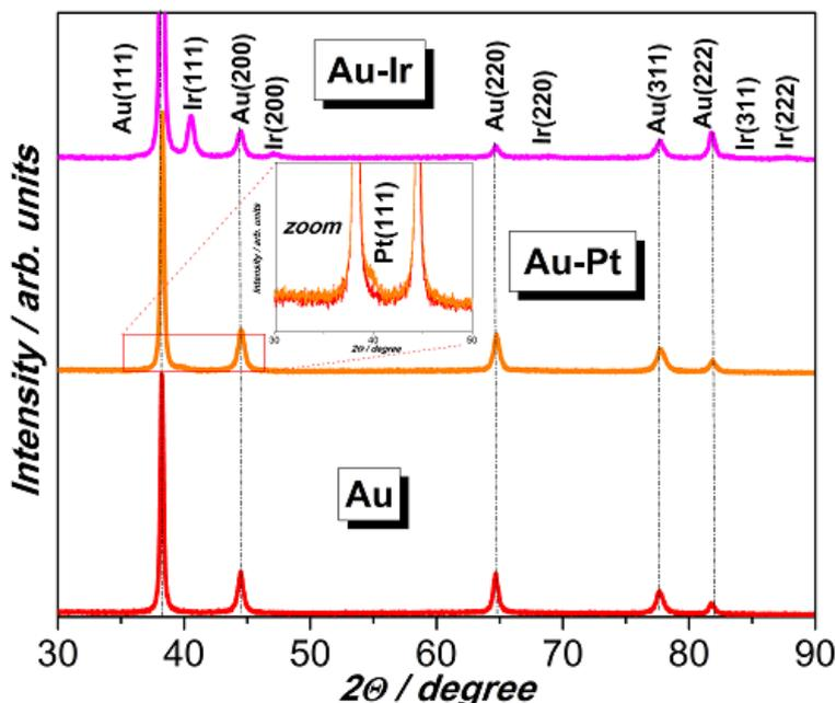
Figure 1. XRD spectra of the Au, Au-Pt and Au-Ir catalytic films.
