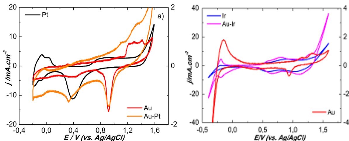
**Figure 3** Cyclic voltammograms of Au-Pt (a) and Au-Ir (b) in 0.5M H<sub>2</sub>SO<sub>4</sub>; potential ranges (a) -0.2 to 1.6 V and (b) -0.4 to 1.6 V; scan rate 100 mV.s<sup>-1</sup>.
