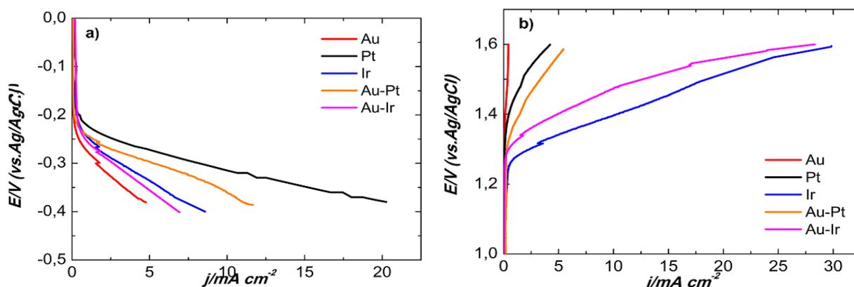
**Figure 4.** Quasi-steady state polarization curves - HER (a) and OER (b) of the sputtered catalytic films in 0.5M H<sub>2</sub>SO<sub>4</sub>; scan rate 1 mV.s<sup>-1</sup>.
