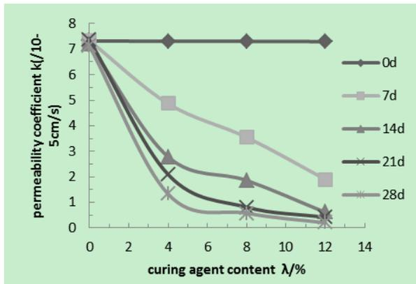
Fig. 4. Relationship between the permeability coefficient and curing agent content.
