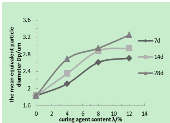
**Fig. 6.** Relationship between the mean equivalent particle diameter and curing agent content.
