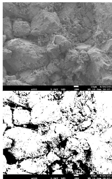
**Fig. 2.** Microscopic imageand binary image of solidified dredger fill
