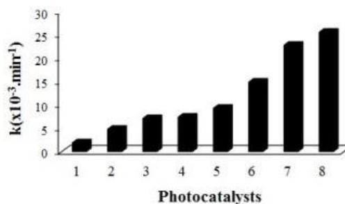
Fig. 5. Comparison data of apparent rate constants of: 1- Al<sub>2</sub>O<sub>3</sub>, RB5; 2- Al<sub>2</sub>O<sub>3</sub>, MG; 3- Ag-Al<sub>2</sub>O<sub>3</sub>, RB5; 4- Ag-Al<sub>2</sub>O<sub>3</sub>, MG; 5- Al<sub>2</sub>O<sub>3</sub>, MCA, RB5; 6- Al<sub>2</sub>O<sub>3</sub>, MCA, MG; 7- Ag-Al<sub>2</sub>O<sub>3</sub>, MCA, MG; 8- Ag-Al<sub>2</sub>O<sub>3</sub>, MCA, RB5 photocatalysts in degradation of RB5 and MG dyes.
