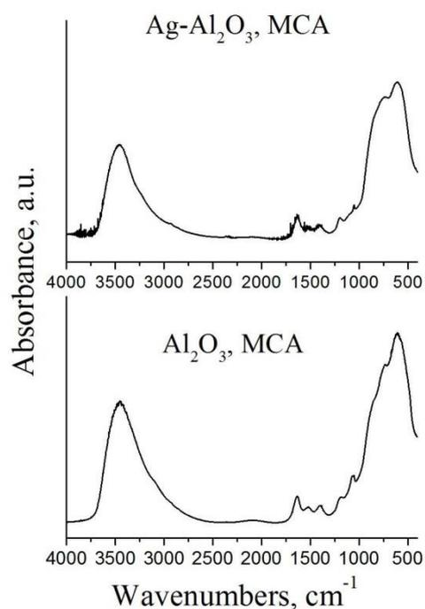
Fig. 2. FT-IR spectra of the studied samples.
