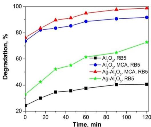
Fig. 4. Degree of degradation of RB5 dye as a function of the time of UV illumination.
