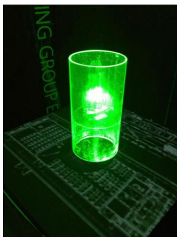
Fig. 5. Holographic display design by combining a cylindrical hologram of a 3D object with its 2D projection mapping.
