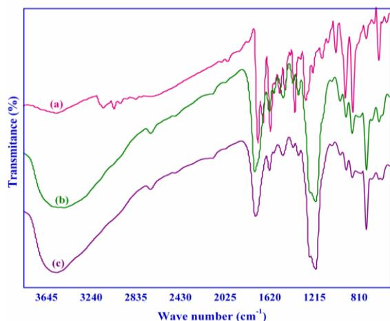
**Fig. 1.** FT-IR spectra of (a) EPDM, (b) BMI and (c) EPDM-g-BMI
