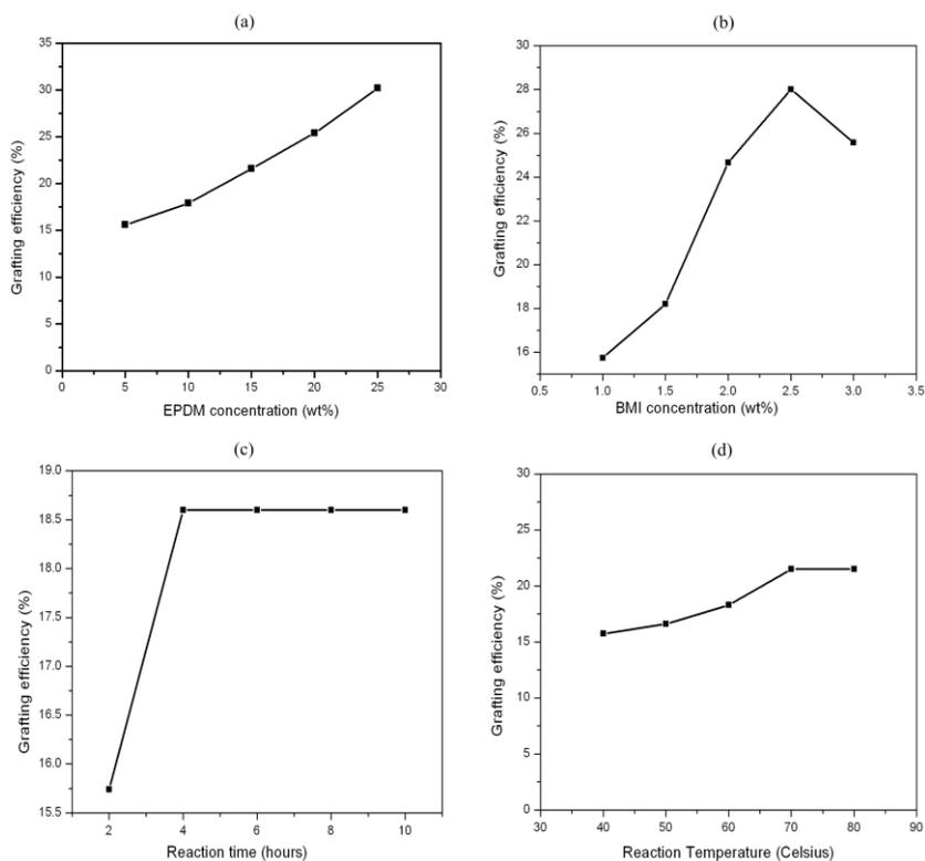
**Fig. 2.** Plot of grafting efficiency against (a) EPDM concentration; (b) BMI concentration; (c) reaction time; (d) reaction temperature.
