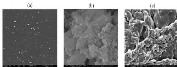
**Fig. 4.** SEM micrograph of (a) EPDM; (b) BMI; (c) EPDM-g-BMI.
