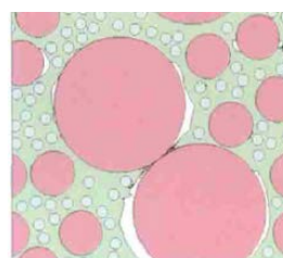
Fig. 3. Cracks under the action of a compressive force.
