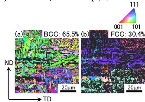
Fig. 3. Diagram orientation of high nickel steel (a) BCC (b) FCC
