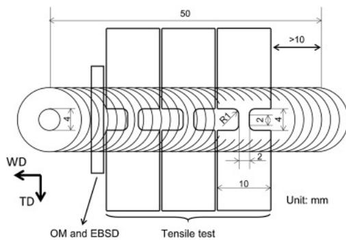
Fig. 2. Geometry and sampling locations of the tensile specimen.
