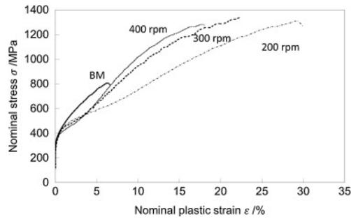
**Fig. 13.** Stress - strain curves of the samples of the parent material and the mixing zone.
