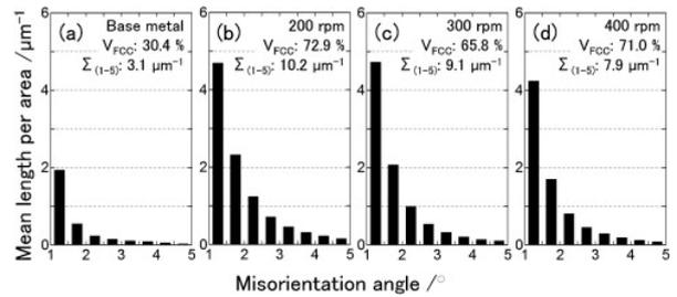
Fig. 11. FCC phase of parent material (a) and stir zone (B, C, d) the proportion of specific bits of the angle histogram.
