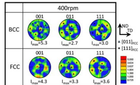
**Fig. 9.** The orientation of the mixing zone of the 400r/min joint with a rotation speed.
