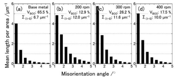
Fig. 12. BCC phase of parent material (a) and stir zone (B, C, d) the proportion of specific bits of the angle histogram.
