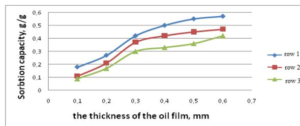
**Fig.3.** Dependence of the sorption capacity of the sorbent on the thickness of the oil film: 1 - rubber foam + carbonizate of sunflower husk (FRCSH- 300); 2- polystyrene foam + carbonizate of rice husk (PFCRH -400); 3- modified rubber foam (MFR-300)
