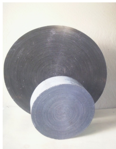
Fig.2. Full-size catalytic neutralizers on block metal carriers
