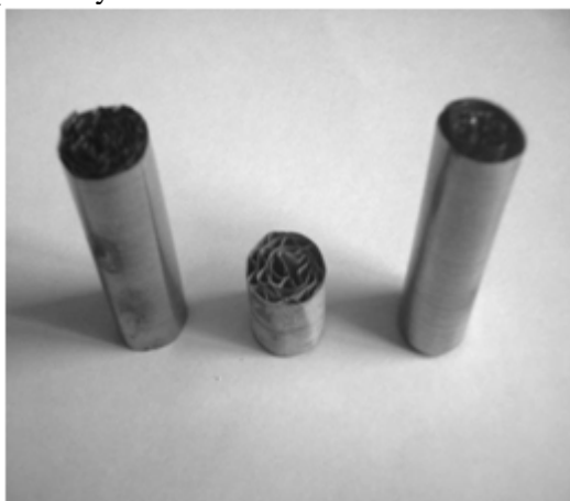
Fig. 1. Laboratory samples of neutralizers on metal blocks
