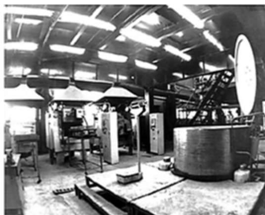
Fig. 3. Centrifuge for impregnating metal on the block carrier
