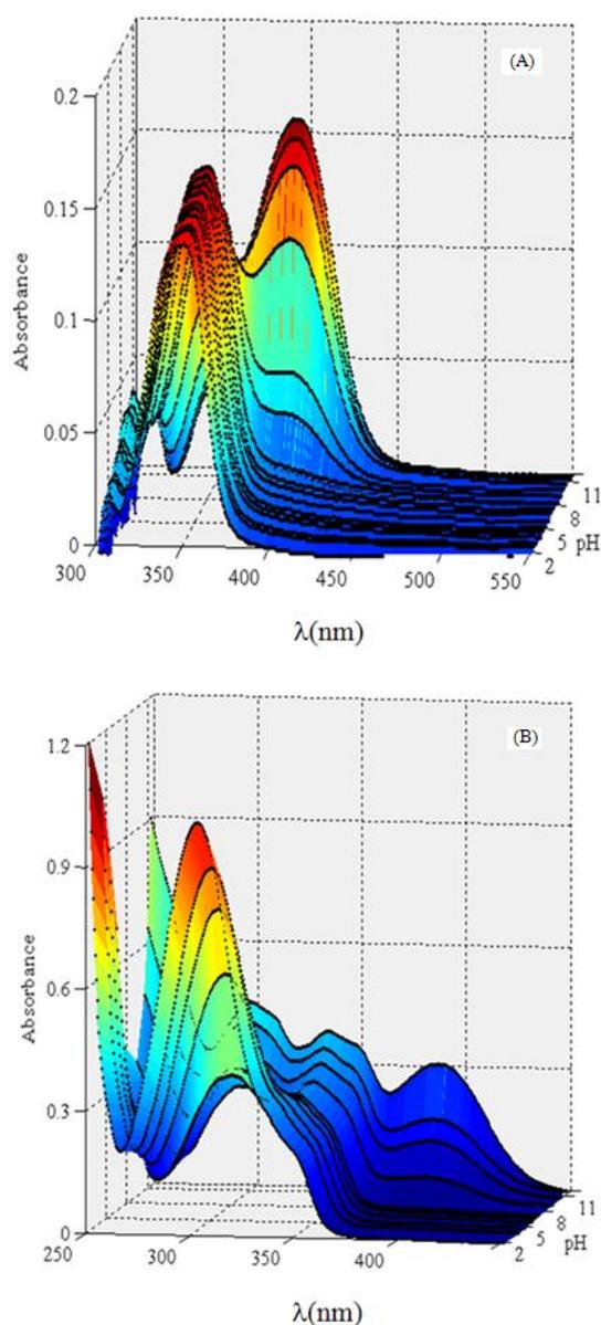
**Fig. 2.** UV-Vis absorption spectra of LH<sub>2</sub> immobilized in photographic film (A) and agarose (B) membranes as a function of pH.
