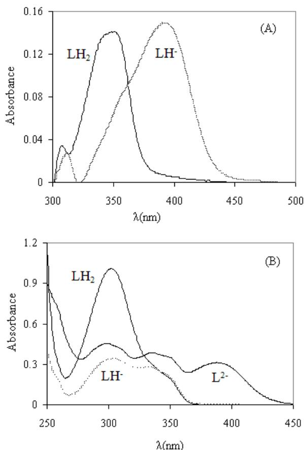
**Fig. 5.** Pure spectra of each assumed species of LH<sub>2</sub> immobilized in photographic film (A) and agarose (B) membranes.
