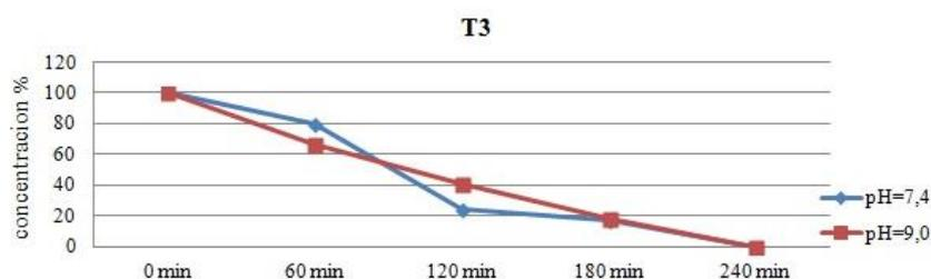
Fig. 10. Hydrolytic stability of T3 after 1 year storage measured at 220 nm by RR-HPLC.
