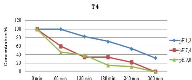
Fig. 7. Hydrolytic stability of T4 on different pH measured at 220 nm by UV –spectroscopy.
