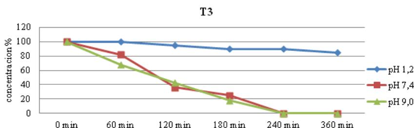
**Fig. 6.** Hydrolytic stability of T3 on different pH measured at 220 nm by UV – spectroscopy.
