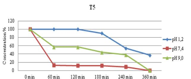
Fig. 8. Hydrolytic stability of T5 on different - pH measured at 220 nm by UV –spectroscopy.
