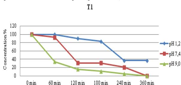
**Fig. 4.** Hydrolytic stability of T1 on different pH measured at 220 nm by UV – spectroscopy.
