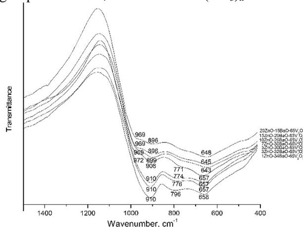
**Fig. 4.** IR spectra of ZnO-BaO-V<sub>2</sub>O<sub>5</sub> glasses.
