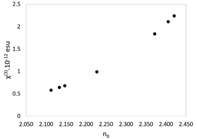
Fig. 6. Third order nonlinear optical susceptibility as a function of refractive index of the glasses.
