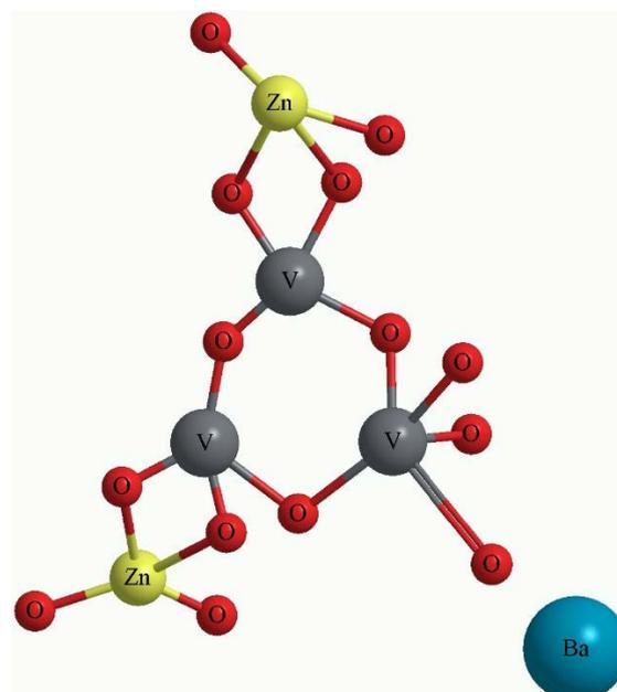
**Fig. 5.** Structural model for glass with high ZnO content.
