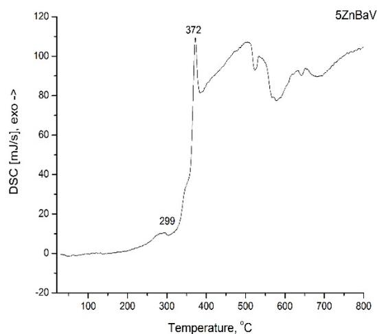
**Fig. 2.** DSC curve of glass with composition 5ZnO.30BaO.65V<sub>2</sub>O<sub>5</sub>.
