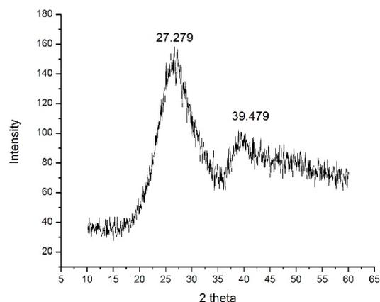
**Fig. 1.** XRD pattern of glass with composition 5ZnO.30BaO.65V<sub>2</sub>O<sub>5</sub>.
