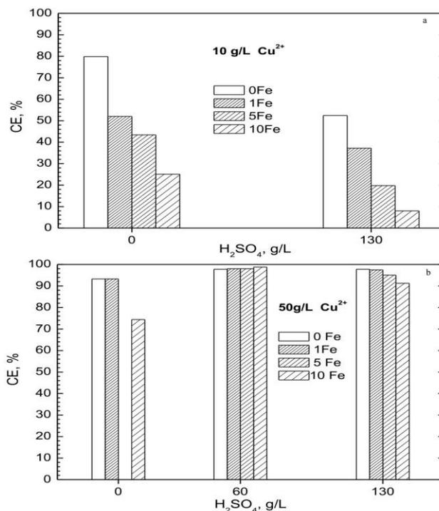
**Fig. 3.** Current efficiency of copper depositions depending on ferrous ion concentration and the presence of free sulfuric acid. Deposition at current density 2.0 A/dm<sup>2</sup> for 5 hours.
