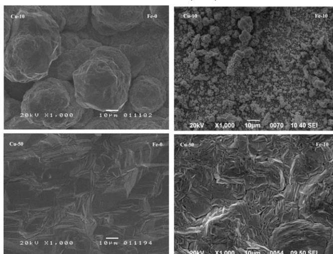
**Fig. 4.** Morphology of deposited copper coatings in the presence and absence of ferrous ions. SEM images x1000, current density 2.0 A/dm<sup>2</sup>, deposition time 5.0 h, free sulphuric acid 130 g/L. Metal ion concentrations shown on pictures in g/L.
