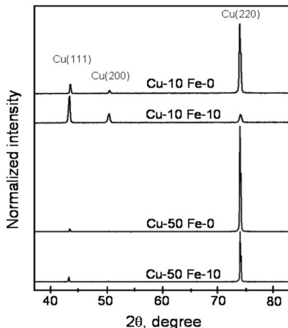
Fig. 5. Powder diffraction analyses of copper samples.
