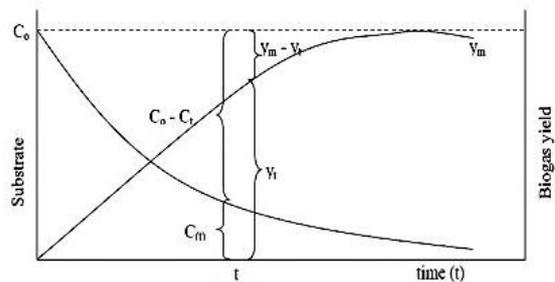
**Fig. 1.** Changes of substrate concentration and rate of gas production
