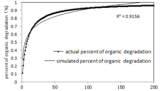
**Fig. 3.** HRT effects on VS degradation rate
