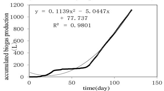
**Fig. 4.** Comparison of accumulated biogas production and model curve
