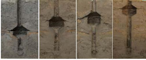
**Fig. 8** Failure behavior after the pile being taken
