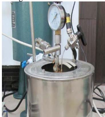
**Fig. 1.** Experimental setup of the safety chemistry of the ClO<sub>2</sub> oxidation of the oil/water transition layer
