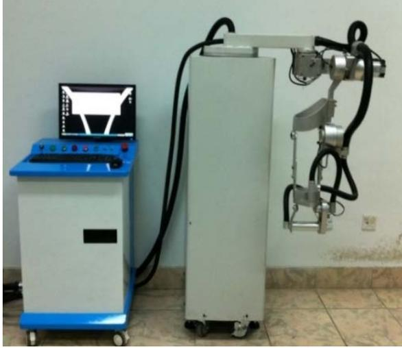
Fig. 1. Rehabilitation robot structure.
