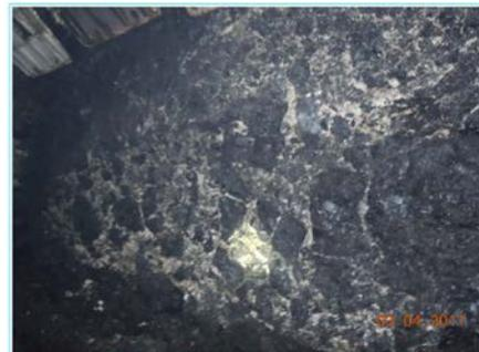
(b) Cementation effect of cutting layer
