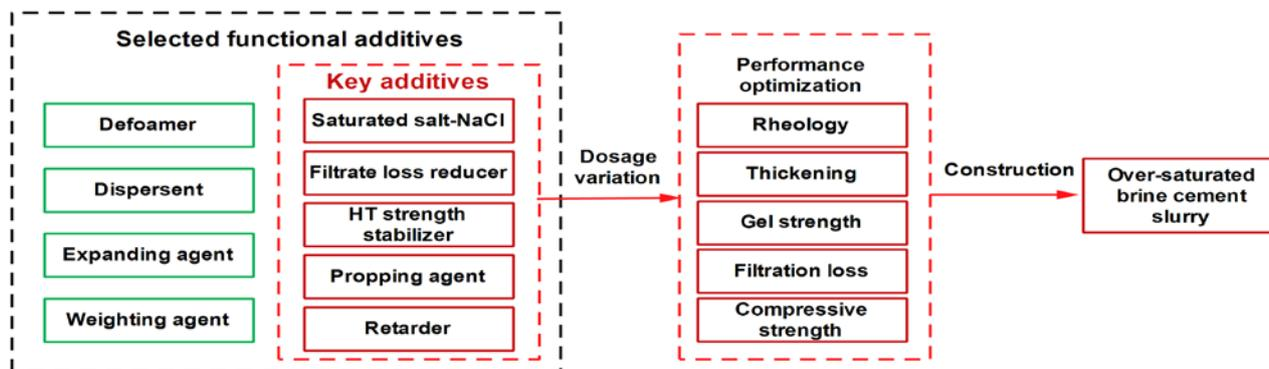
**Fig. 1.** Experimental design of constructing over-saturated brine cement slurry.
