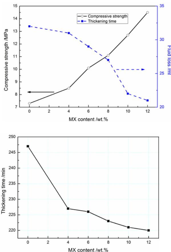
**Fig. 6.** upper: relation between MX content and compressive strength and fluid loss; lower: relation of MX content vs. thickening time.
