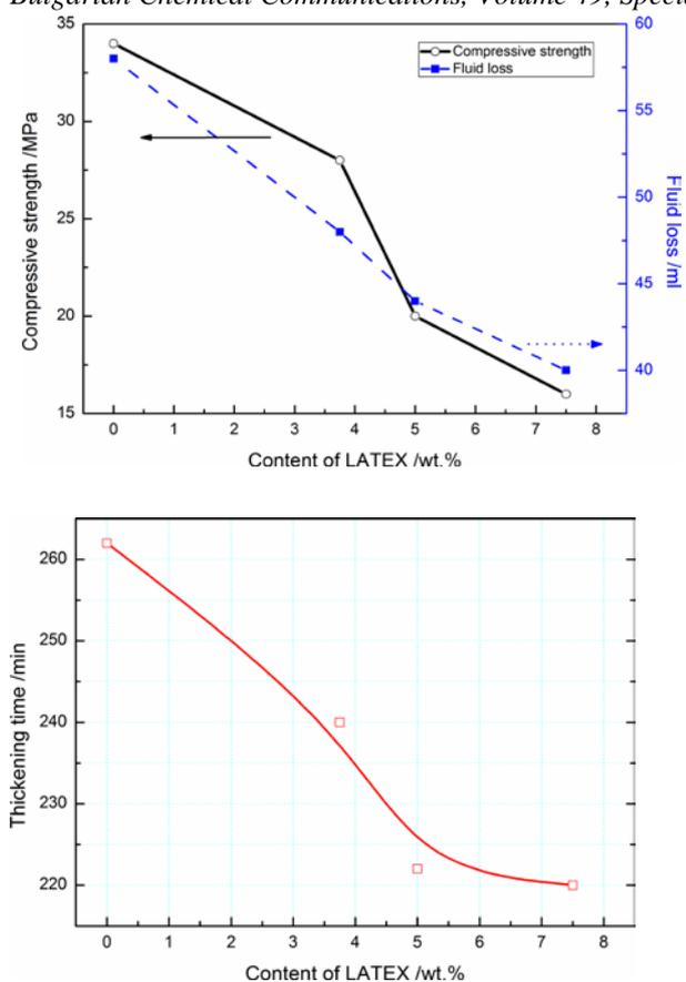
**Fig. 2.** upper: relation between content of LATEX and compressive strength and fluid loss; lower: curve of content of LATEX vs. thickening time.
