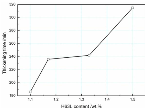
**Fig. 5.** Relation between H63L content and thickening time.
