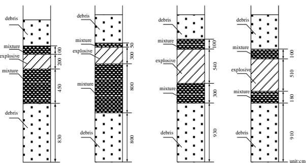
Fig. 7. Charging results in the dry borehole
