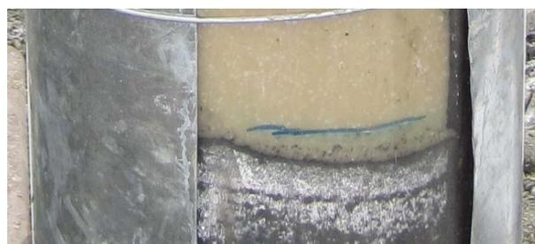
**Fig. 13.** Charging experiments of the mixed emulsion explosive in water-filled borehole models with isolators
