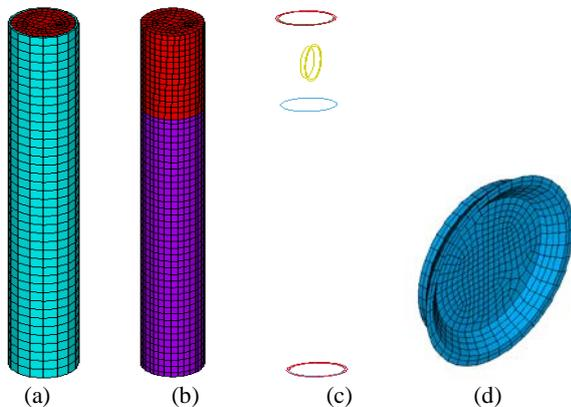
Fig. 2. Calculation models and finite element grids
