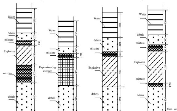
Fig. 8. Charging results in the water borehole
