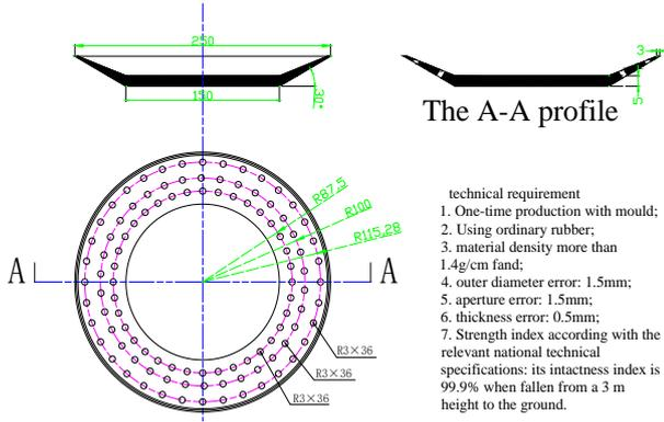
Fig. 1. Plate-shaped MEE-rock debris isolator
