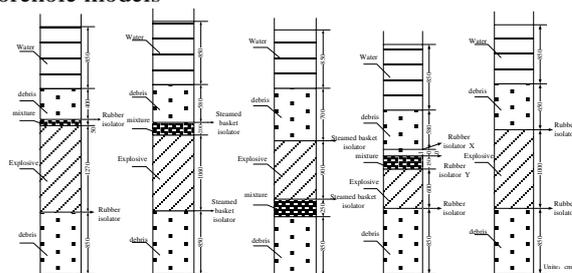
**Fig. 12.** Structures of charging experiments in water-filled borehole models
