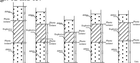
**Fig. 11.** Structures of charging experiments in dry borehole models
