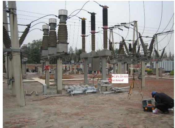
Fig. 8. A photo of the field experiment on the electromagnetic disturbance of a wireless sensor
