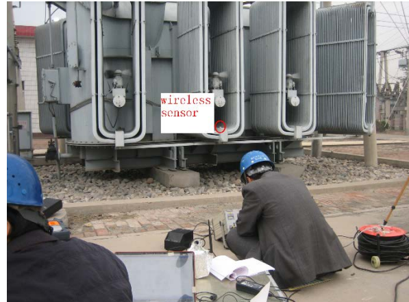
Fig. 18. A photo of the field experiment on communication obstruction of a wireless sensor
