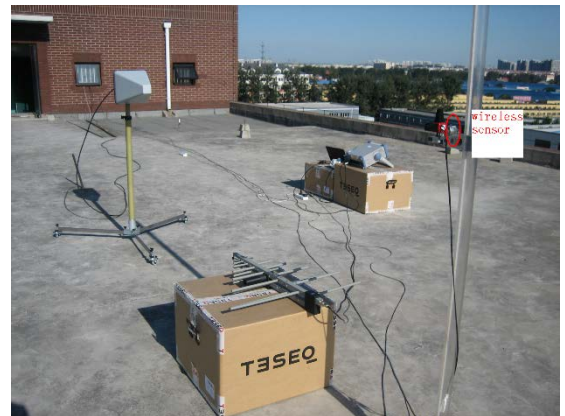
Fig. 9. Photo of immunity test on the wireless sensor performed at an open area test site
