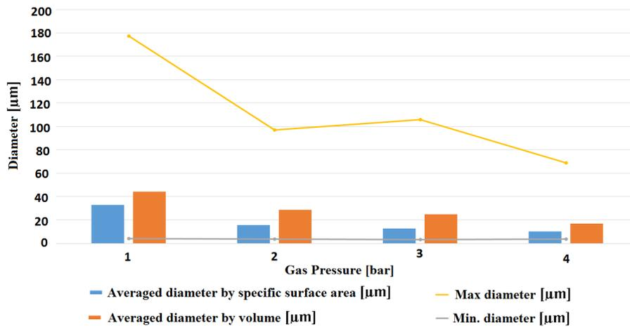
**Fig. 4.** Summarized results for the minimum and the maximum diameters detected, averaged diameters by specific surface area and by volume, for different gas pressures (1-4 bar), for the automated system for fog generation, at a spraying distance of 65 cm
