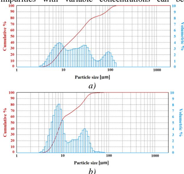
**Fig.5.** Diameter distribution and amount of droplets of: a) pure distilled water; b) distilled water + 5% KH<sub>2</sub>PO<sub>4</sub>.
