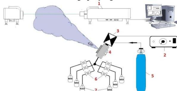
**Fig. 2.** Block diagram of the automated system for generation of fog with impurities – (1) laser particle size analyzer; (2) spray duration control unit; (3) electromagnetic valve; (4) nozzle; (5) pressurized gas tank; (6) valves; (7) fluid containers
