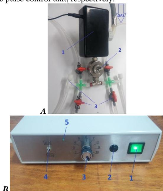
**Fig. 1. A.** Fog spraying unit: (1) electromagnetic valve; (2) fog generating nozzle (orifice diameter of 0.4 mm); (3) valves; **B.** Control unit: (1) power button; (2) pulse initiation button; (3) knob for setting the timer (seconds); (4) switch for selection of time multiplier; (5) LED indicator for operation
