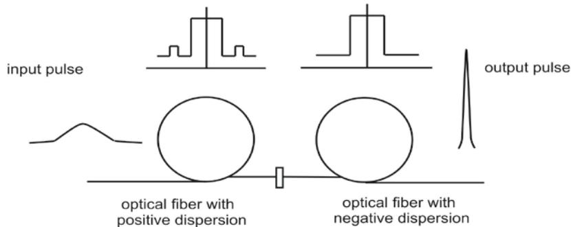
Fig. 1. Improved multisoliton compressor
