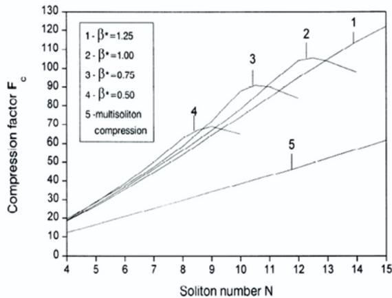
**Fig. 3.** Compression factor  $F_c$  versus the soliton number  $N$ .
