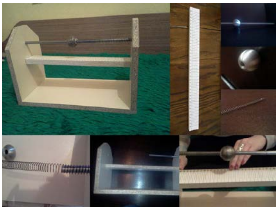
Fig. 1. A device for demonstrating harmonic oscillation and for measuring the deviation of an oscillating body.
