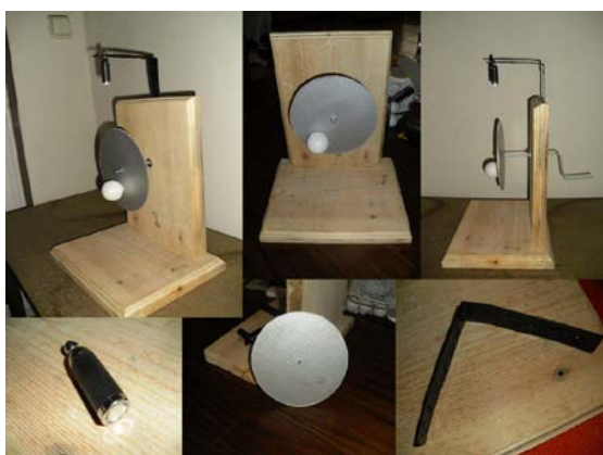
Fig. 2. A device establishing the analogy between harmonic oscillation and moving in a circle.
