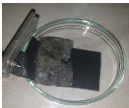
Fig. 2. Anodic biofilm formed during prolonged operation of MFC (K1) under load (1 \text{k}\Omega ).
