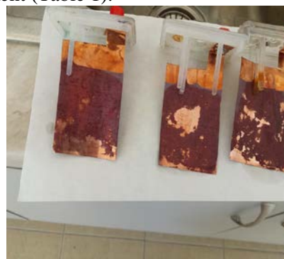
Fig. 4. Deposition of copper on cathodes after operation of microbial fuel cells at constant load (1 \text{k}\Omega ).
