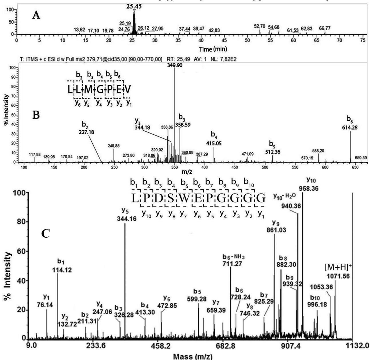
**Figure 1.** A) Extracted chromatogram, B) MS<sup>2</sup> fragmentation of LLMGPEV peptide with m/z 379.17 [M+2H]<sup>2+</sup>, C) MALDI-MS spectrum (positive ion mode) of the peptide at m/z 1071.56[M+H]<sup>+</sup>. Standard peptide solution was used to calibrate the mass scale of the Autoflex<sup>TM</sup> III, High Performance MALDI-TOF & TOF/TOF Systems (Bruker Daltonics).
