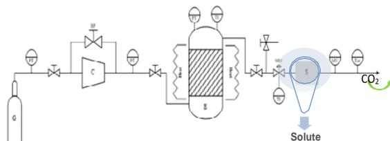
**Fig. 1.** Diagram of the supercritical fluid extraction apparatus. G, CO<sub>2</sub>; C, compressor; E, extractor; S, separator; BP, back-pressure regulator; MM, micrometer valve; MV, flow meter; Tot, totalizer; TI, temperature indicator, PT, pressure indicator.
