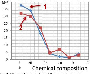
**Fig.2.** Chemical composition of the surfacing powder 1- Powder alloyPG-Z40 – 100%;
