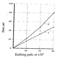
**Fig.6.** The new alloy and steel wear rates: 1-The new PG-Z40+10% CrB<sub>2</sub> alloy 2-45 steel, 55 HRC hardness
