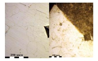
Fig.4.The size of an impression on the polished specimen of the samples: a) PG-Z40; b) PG-Z40+10%  $CrB_2$
