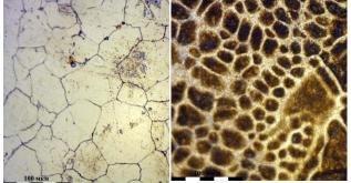
X500 magnification Fig.7. Microstructure of the layer surfaced with PG-Z40 alloy (a) and PG-Z40+10% CrB<sub>2</sub> alloy
