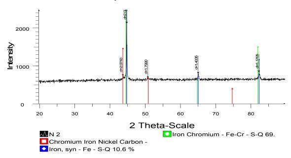
Fig.3. The results of X-ray structure analysis for PG-Z40+10% CrB<sub>2</sub>
