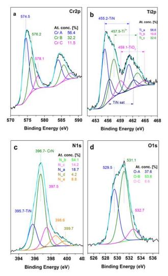
**Fig.9.** XPS spectra of CrN/TiN multilayer coating (a) Cr2p, (b)- Ti 2p, (c)- N 1s and (d) O 1s
