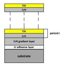
Fig.1. A principal scheme of the multilayer CrN/TiN coating
