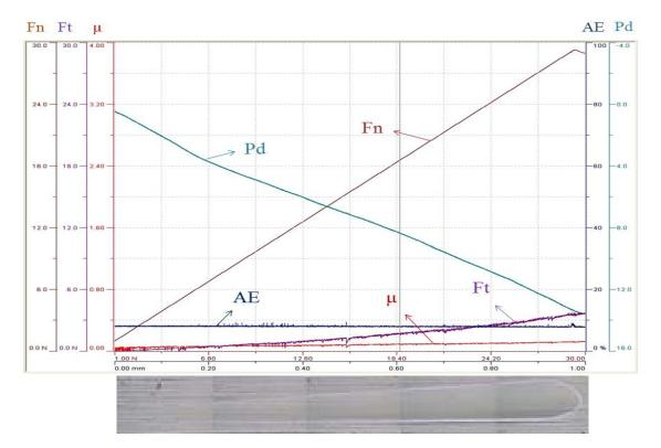
**Fig.6.** Optical image of the scratch track in the CrN/TiN coating and scratch test results of the normal force (Fn), penetration depth (Pd), acoustic emission (AE), friction force (Ft) and coefficient of friction ( $\mu$ )
