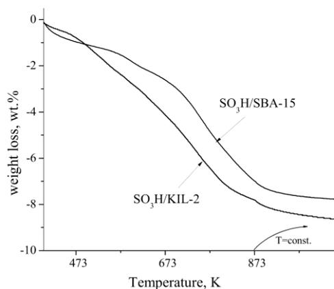
Fig. 2. TGA of SO<sub>3</sub>H/SBA-15 and SO<sub>3</sub>H/KIL-2 samples.
