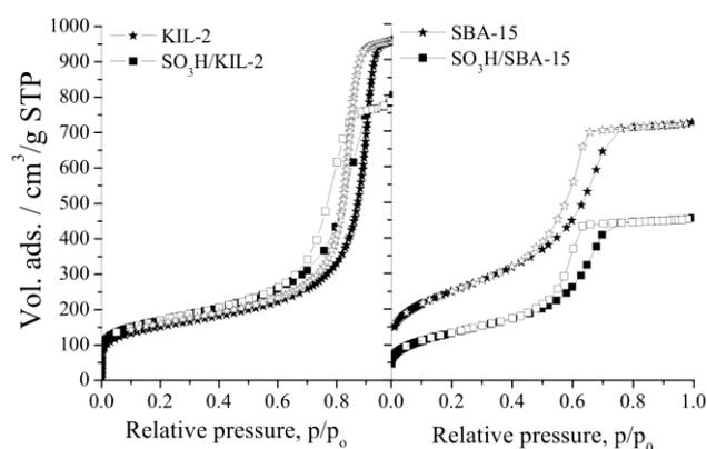
Fig. 1. Nitrogen adsorption/desorption isotherms of SBA-15 and KIL-2 silicas and their sulphonic analogues.
