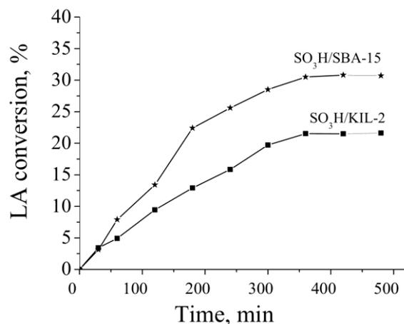
Fig. 4. Catalytic activity of  $\text{SO}_3\text{H/SBA-15}$  and  $\text{SO}_3\text{H/KIL-2}$  samples in levulinic acid esterification with ethanol at 343 K.
