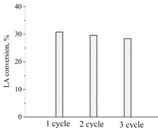
Fig. 5. Catalytic activity of  $\text{SO}_3\text{H/SBA-15}$  sample.
