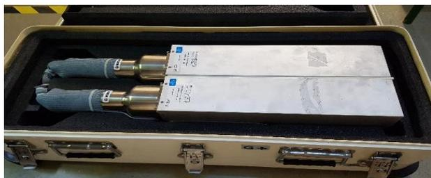
**Fig. 1.** Opened detector protection box, keeping a pair of NaI(Tl) detectors used in the survey.
