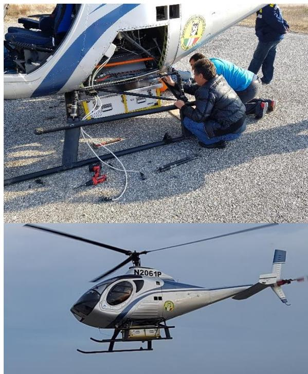
**Fig. 2.** The spectrometry system installed on Schweizer 333 (269D).
