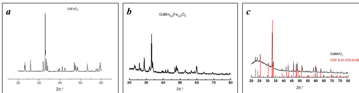
Figure 1. XDR patterns of complex oxides: (a) GdFeO<sub>3</sub>; (b) GdMnO<sub>3</sub>; (c) GdMn<sub>0.5</sub>Fe<sub>0.5</sub>O<sub>3</sub>
