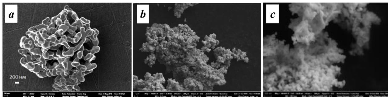
Figure 2. SEM images of GdFe<sub>1-x</sub>Mn<sub>x</sub>O<sub>3</sub> complex oxide: (a) x=0, (b) x=0.5, (c) x=1
