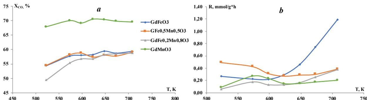
Figure 3. Temperature dependence of (a) the CO conversion and (b) the rate of formation of CO<sub>2</sub> (at a ratio of CO:H<sub>2</sub> = 1:2)
