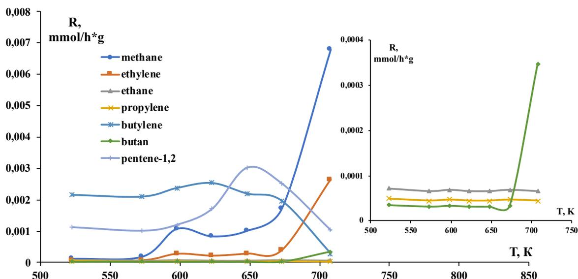
Figure 4. The temperature dependences of the hydrocarbons formation rates over GdMnO<sub>3</sub> (at ratio of CO:H<sub>2</sub>=1:2)
