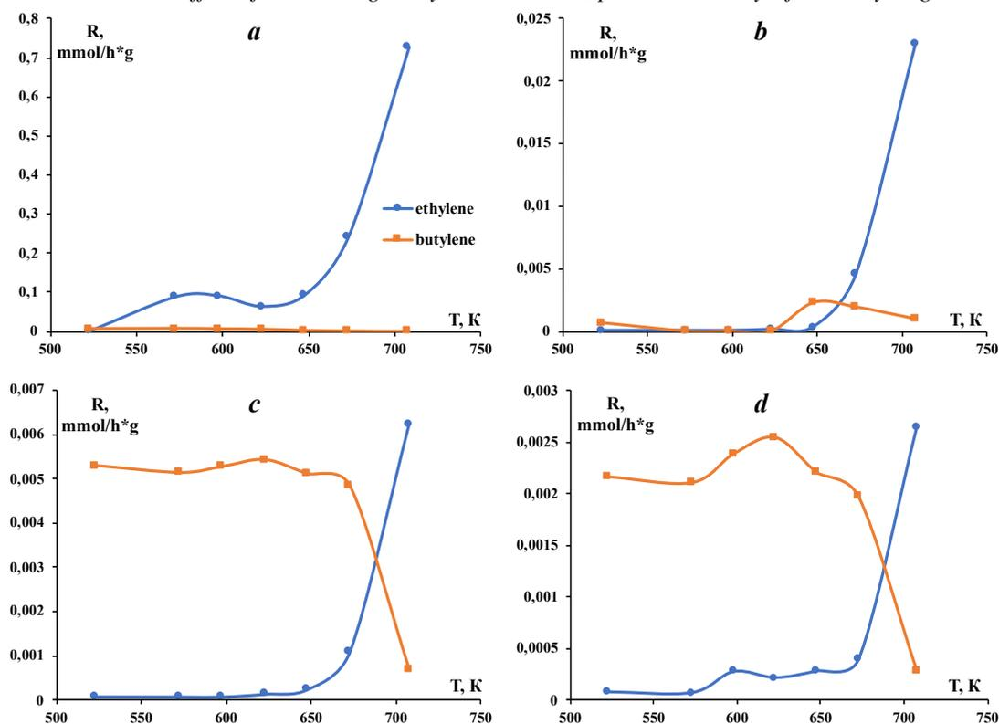
**Figure 5.** The temperature dependences of ethylene and butylene production rates over GdFe<sub>1-x</sub>Mn<sub>x</sub>O<sub>3</sub> perovskite catalysts: (a) x=0, (b) x=0.5, (c) x=0.8, (d) x=1
