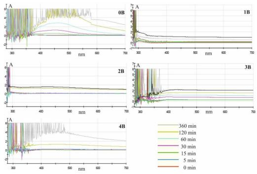
Figure 2. UV-Vis studies of the formation of AgNPs with time. The sample numbers are according to Table 1.
