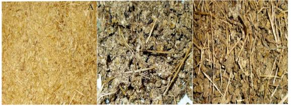
**Figure 1.** Chamomile wastes investigated: A. after extraction with 1,1,1,2-tetrafluoroethane (F); B. after hydrodistillation (HD); C. after steam distillation (S)
