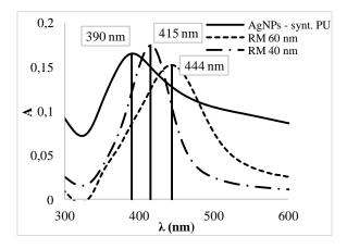
**Fig. 1**. UV-vis spectra of nanocolloidal suspensions from two RMs of AgNPs 60nm and 40nm and AgNPs synthesized in our lab.
