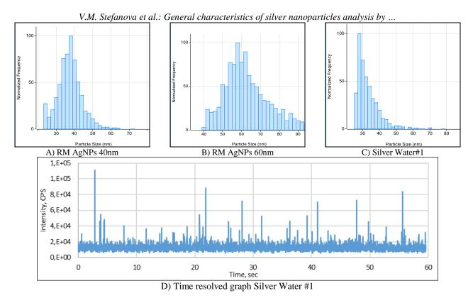
Fig. 3. Size distribution diagram of A) RM AgNPs 40 nm; B) RM AgNPs 60 nm; C) Silver water#1 and D) timeresolved data record for Silver water #1
